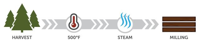
Developed in Finland, and successfully used commercially in Europe since the 1990's, Thermal Modification is a chemical free method of heat treating wood with nothing more than steam and high temperatures in order to increase the woods water repellency, insect and rot resistance and dimensional stability.
